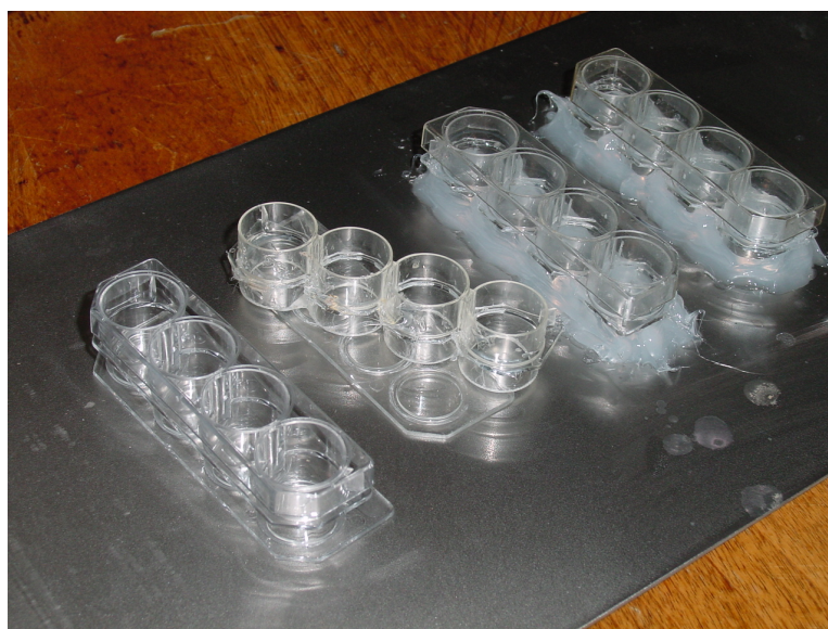
Figure 2.5: Sonicseal Wells. [As from the factory (left), removed from their base (left center), and affixed to a plate (right, 2)]
